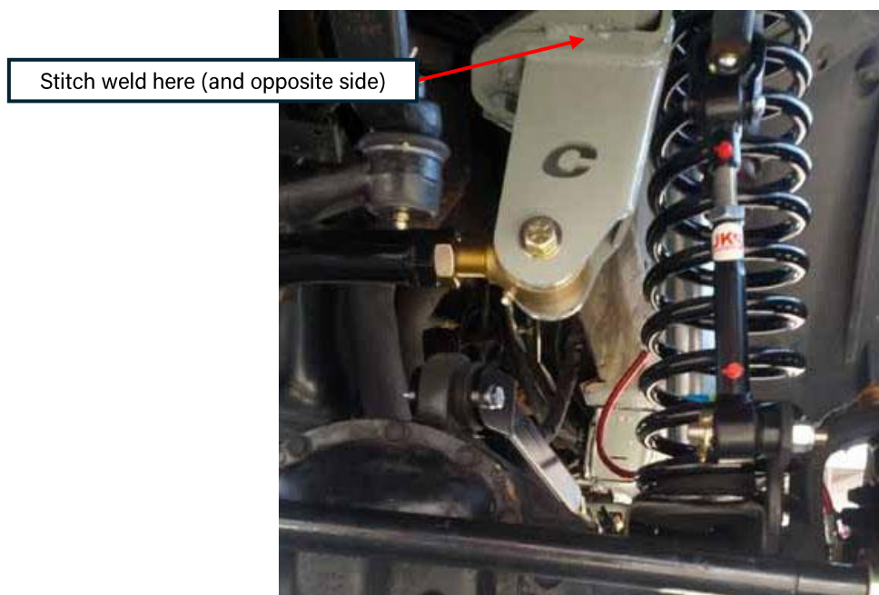
XJ frame-side bracket weld locations
