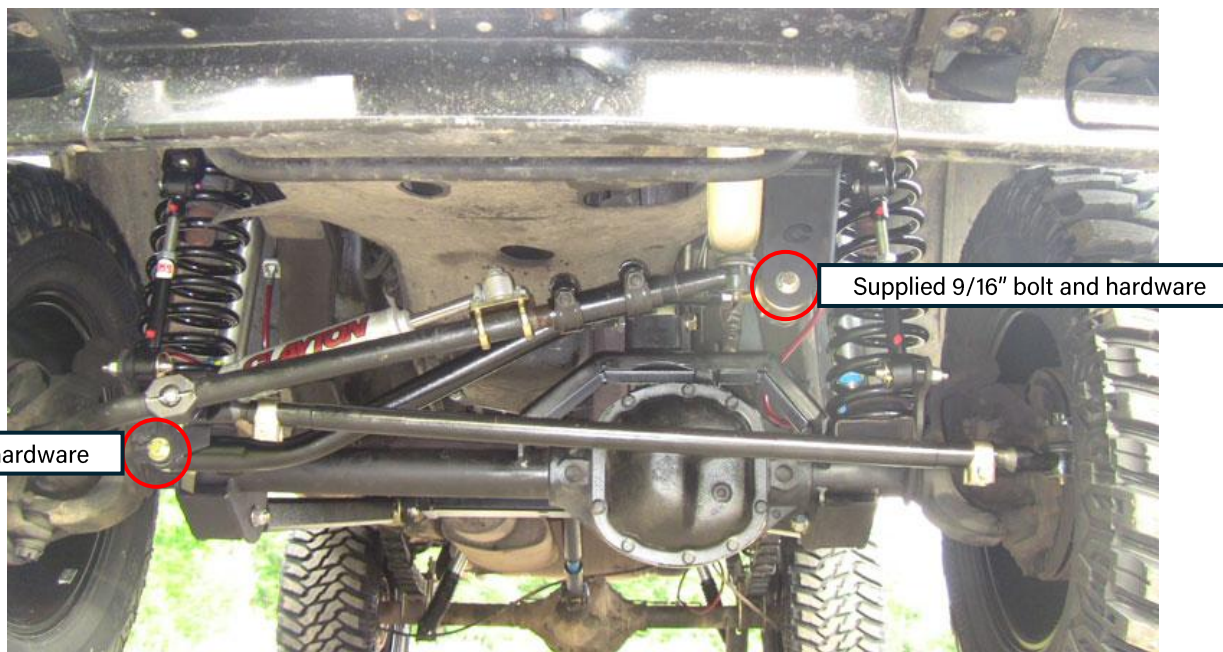
XJ bracket and track bar fully installed and painted
