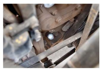
**STEP 2** Remove dipstick bracket hardware.
