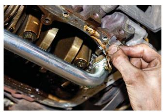
**STEP 6** Re-install the dip stick into the block.
