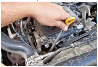
**STEP 5** Place freeze plug in stock dipstick hole.
