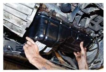
**STEP 17** Install the drain plug with gasket.
