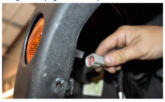
4. Remove the plastic fender/flare support. You may need to remove more hex head bolts and/or plastic retainer clips.
