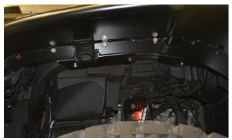
Observe how the Crusher Flare sits into the pocket in the fender sheet metal, and make any necessary adjustments to ensure that it is perfectly aligned as the hardware is tightened. The goal is to maintain a uniform gap along the top of the Crusher Flare where it sits into the fender pocket, from front to back.
