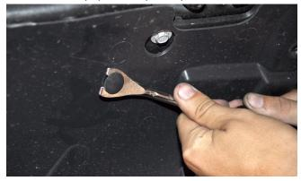
Try not to damage the inner fender or the plastic retainers. Set the inner fender, all of the plastic retainers and hex head bolts aside, as some will be re-used during the installation process.
