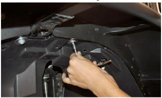
**28.** At the rearward edge of the inner fender liner, mark where the holes in the "L" brackets are located behind the inner fender.
