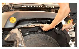
**3.** Disconnect the side marker lamp by pulling the wiring harness plug out of the lamp socket.
