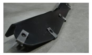
7. Align the Upper Sub-Frame Bracket as shown in figure 22, and slide it upward between the outer fender sheet metal and the inner tub brace. It may be a tight fit, and could require a firm shove or two. Position it so that the threads of the u-nuts are roughly aligned with the 5 corresponding holes in the outer fender.
