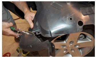
Once the large parts are out of the way, test-fit the inner fender again and make marks for more fine-tuned trimming. It should take several of these steps to finally get it right. Just be sure not to cut away too much in any step, be patient and you will eventually get it just right.
