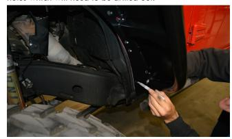
Use a scribe to mark along the fender sheetmetal that extends into the wheel opening, beyond the mounting plate of the Crusher Flare, both at the back of the wheel opening...
