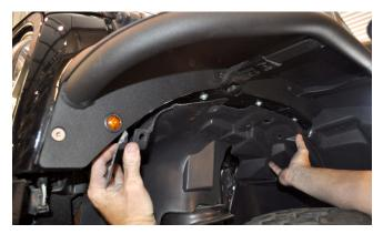
27. Once the inner fender liner is trimmed to fit, attach it by first removing the two previously-installed bolts from Upper Sub-Frame Bracket that appear through the access holes in the inner fender liner. Remove each of these bolts, place one of the provided 5/16 fender washers under the head of each, then re-install and tighten.
