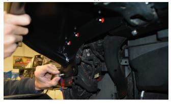
Continue installing hardware into the remaining available holes. Note the following diagram which shows the locations to use the 1" long flat head cap screws. The remaining holes get the 3/4" long flat head cap screws. (Note: several of the hole locations will need to be drilled out, and will not be able to accept hardware yet—leave these holes unused at this time.)
