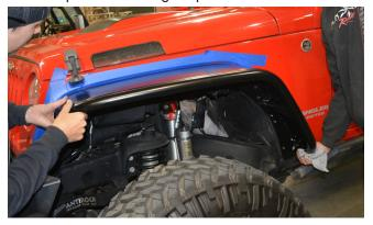
Install two of the 5/16-18 X 3/4 stainless steel flat head cap screws, one at the rear and one at the front end of the Crusher Flare. The one at the front will need to be backed by a flat washer and lock nut (supplied in the hardware kit)
