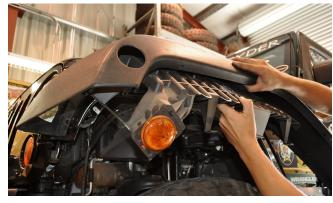
Remove the stock fender flare. There will be several more plastic retainer clips to remove in order to remove the flare.
