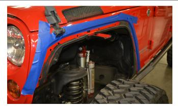
9. Pre-install the Crusher Flare. Place it against the Jeep and line up the bolt holes. It will rest somewhat on the stock fender brace to make this task easier. Even with masking tape in place, be careful while handling the Crusher Flare, to keep it from contacting the exterior finish of the Jeep and scratching the paint.
