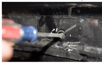
**20.** Re-install the Lower Sub-Frame Bracket. Use two 5/16-18 X 3/4 hex head cap screws with flat washers and nylon insert lock nuts to attach the bracket to the inner tub brace. Keep the holes in the bracket properly aligned with the holes in the outer fender as you tighten the bolts.
