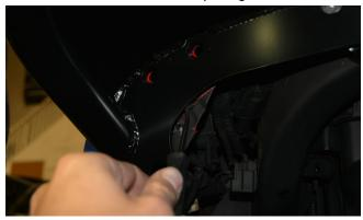
11. Remove the Crusher Flare AND the Upper Sub-Frame Bracket from the Jeep. You'll now see the marks you made for drilling the extra mounting holes and trimming sheet metal around the wheel opening.
