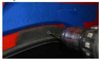
Once all of the pilot holes are drilled, switch to the 21/64" bit and re-drill each hole out to its final size. Be careful when drilling, as the larger bit may want to grab the thin sheet metal and deform it. After the holes are drilled, apply some touch-up paint or clear coat to the bare metal of the hole edges to protect them from rust.
