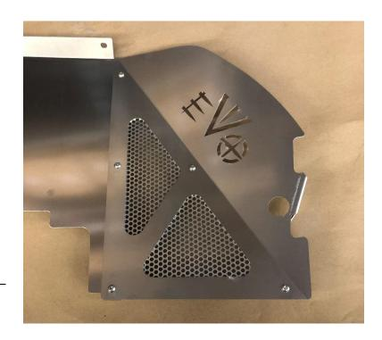
3. Using four more of the supplied #10 bolts and lock nuts (2 for coilover and double throwdown) attach the mid-rear piece overtop of the middle piece then bolt together.
