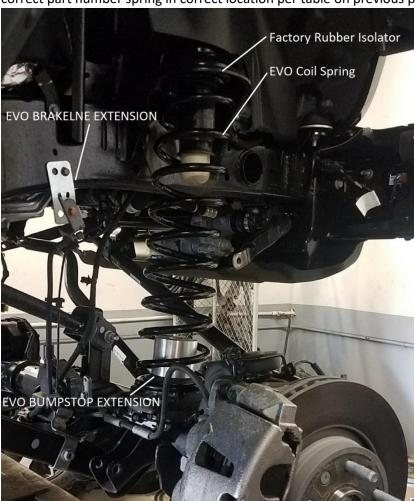
14. With spring in place and bumpstop extension sitting on axle pad and bolt inserted into bumpstop extension. Install supplied 3/8" nut from under spring pad to bolt inserted inside bumpstop extension and tighten.
