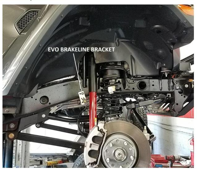
16. Install factory brake line to the new lower location on the EVO brake line extension bracket. Be very careful moving line into new location. The factory hardline will need to be slightly manipulated to be relocated. Do not use tools or pinch/crack the line.
