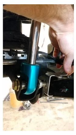
17. Reinstall shock at axle per factory specifications. If you are installing shock extensions. Do so at this time. Follow instructions for that kit. If you are installing new shocks, install shocks at both upper and lower mounting locations. Torque to factory specifications.
