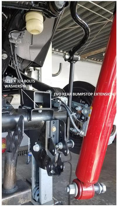
33. Lightly jack front driver side axle tube slightly. With axle slightly supported remove front lower shock bolt from axle. Varying axle jack tension to the right amount will alleviate load on the bolt and allow it to freely slide out. If you are replacing shocks and not using shock extensions remove upper bolt and remove shock. Otherwise leave shock mounted at upper. Support driver side axle with jack stand and repeat this step on passenger side.
