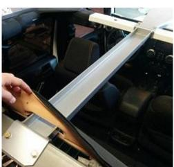
10. After fully tightening the Rear Bar to the C-pillar cross bar, reinstall the dome light and zip the fabric cover back up.
