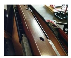
3. With the holes drilled in the factory B-pillar crossbar and front Center Bar in place, lay the rear bar in place, channel up, over the top of the front center bar and align the holes with those on the center bar. Stacking
