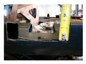
38. Connect your marks and carefully make your cuts. Be very careful not to cut the wiring in the rear of the bar. Depending on the year, it may be wrapped in foam (pictured) or may be exposed. <u>Make shallow cuts to avoid damaging this wiring</u>.
