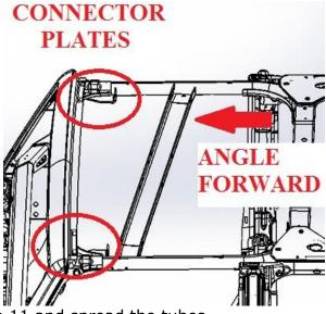
29. Slide the Upper Cross Bar back into place and reinstall the Center Bar. 1<sup>st</sup> thread 2 of the supplied 3" bolts, washers and locknuts through the holes drilled and the outer bolt plate on the crossbar. With these threaded, thread the supplied
