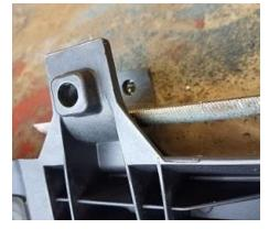
46. Install the door surrounds and verify the fit. If necessary, sand/file again(this may require multiple iterations to achieve an acceptably fit). Note: depending on the holes drilled through the tubes, the C-mount may need to be clearanced around the bolts/washer.
