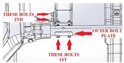
1" bolts through the connector plates. <u>Note: If you have a soft top, it is</u> <u>highly recommended to clearance the inside of the door surround C-mount to</u> <u>fit the bolt plate. This can be done with a file, barrel sander or similar tool. If</u> <u>you choose not to clearance the C-mount, then do not install the outer bolt</u> <u>plate. This process is detailed on last page of these instructions.</u>
