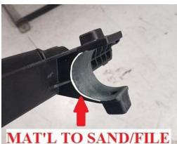
45. Remove the door surrounds and use either a barrel sander or a coarse round/crescent file to remove the material marked in the previous step.
