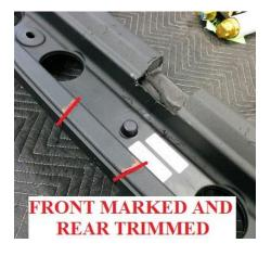
37. With the top of the sound bar marked, measure and mark 1 3/8" down from the top of the sound bar on both sides.
