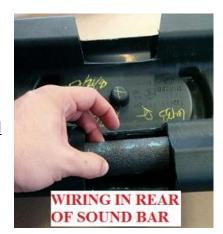
39. Replace sound bar. Verify that the trimmed sound bar fits. If not, mark where additional trimming is needed, remove the sound bar and make the necessary adjustments.
