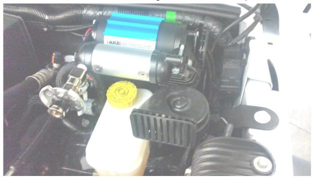
NOTE: Newer Jeep JK models are equipped with a second horn that will require relocating. EVO MFG has made revisions to our bracket to relocate the second horn. If your bracket does not have the revision, you can easily add the horn relocation yourself by using the provided measurements in the photo as well as a drill with a 1/4" drill bit.
