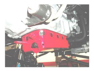
Begin to thread BY HAND all factory bolts into engine through both the EVO Skid and factory oil pan holes. Make sure to thread all bolts in at least 3 full turns on each bolt before using a wrench. You
