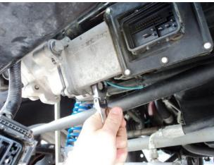
3. Remove factory swaybar actuator. With a screwdriver push into circular chamber and verify the actuator movement.
