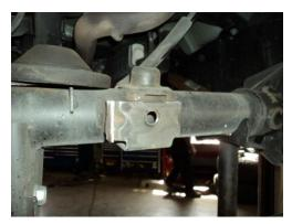
5. Install rear trackbar bracket as shown with supplied 9/16 bolt and U-bolts (make sure to use the locking nuts on the U-bolts).
