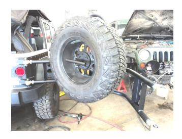
17. Slide T handle through the center hole of the wheel mounting plate and tread into tire carrier.
