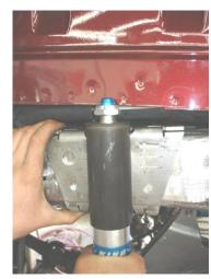
16. With airbumps installed in can, Cycle suspension with tires on and off up and down and make sure this is the correct location and nothing is making inappropriate contact. This is your last chance to make sure it is correct.
