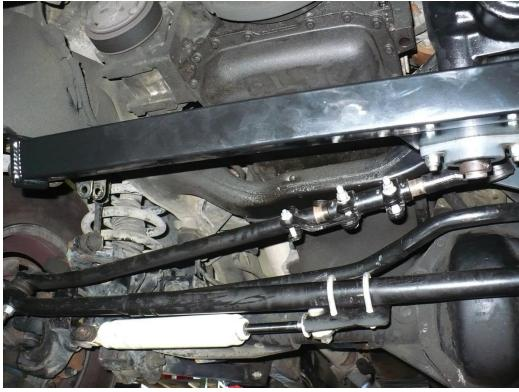
8) Recheck bolts / torques after 100 miles of driving. Grease bearing at normal chassis service intervals.
