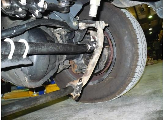
2) Next remove the pitman arm nut on the steering box and install the Pitman arm stud provided in the kit along with the new lock washer provided. Torque to 185 ft-lbs.
