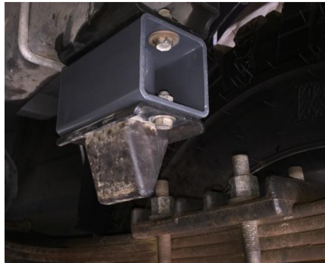
Figure 2. 8520 Dodge Rear Bump Stop Spacers installed on factory mounts.
