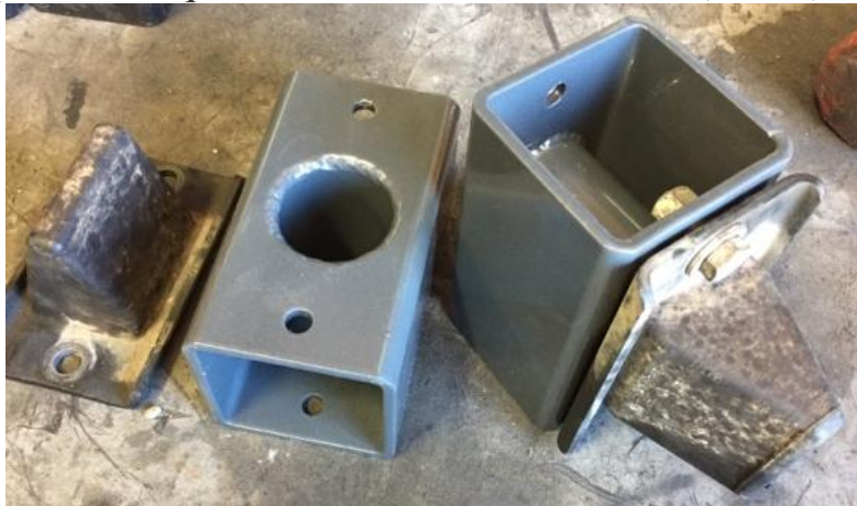
Figure 1. Factory bump stop attached to 8520 Dodge Rear Bump Stop Spacer
