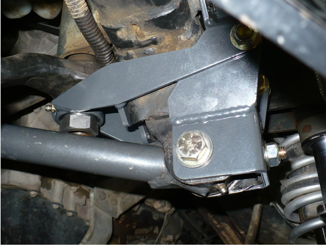
8075 Synergy Manufacturing front track bar at full bump with no bump stop spacers.
