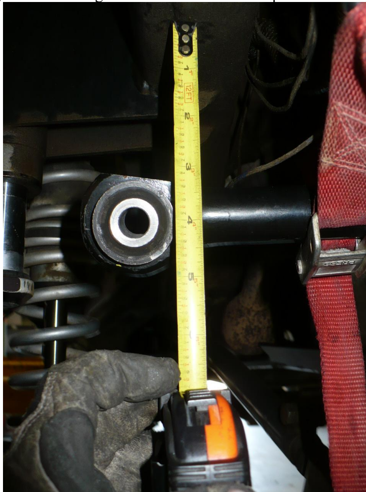
8075 Synergy Manufacturing front track bar at full bump with no bump stop spacers.
