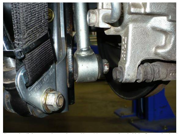
4) Install sway bar link to sway bar as shown. Use a 14mm wrench to hold the flats on the tie rod end stud and a 15mm wrench to tighten the nut. Torque to 50 ft-lbs.
