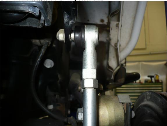
5) With vehicle set at ride height, set tie rod end joint to neutral and tighten tie rod end jam nut. Use two <sup>3</sup>/<sub>4</sub>" wrenches and snug jam nut against tie rod end.
