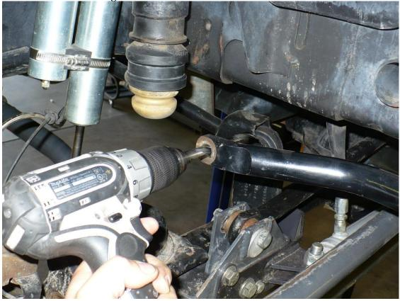
Figure 1. Drilling Out the Sway Bar
