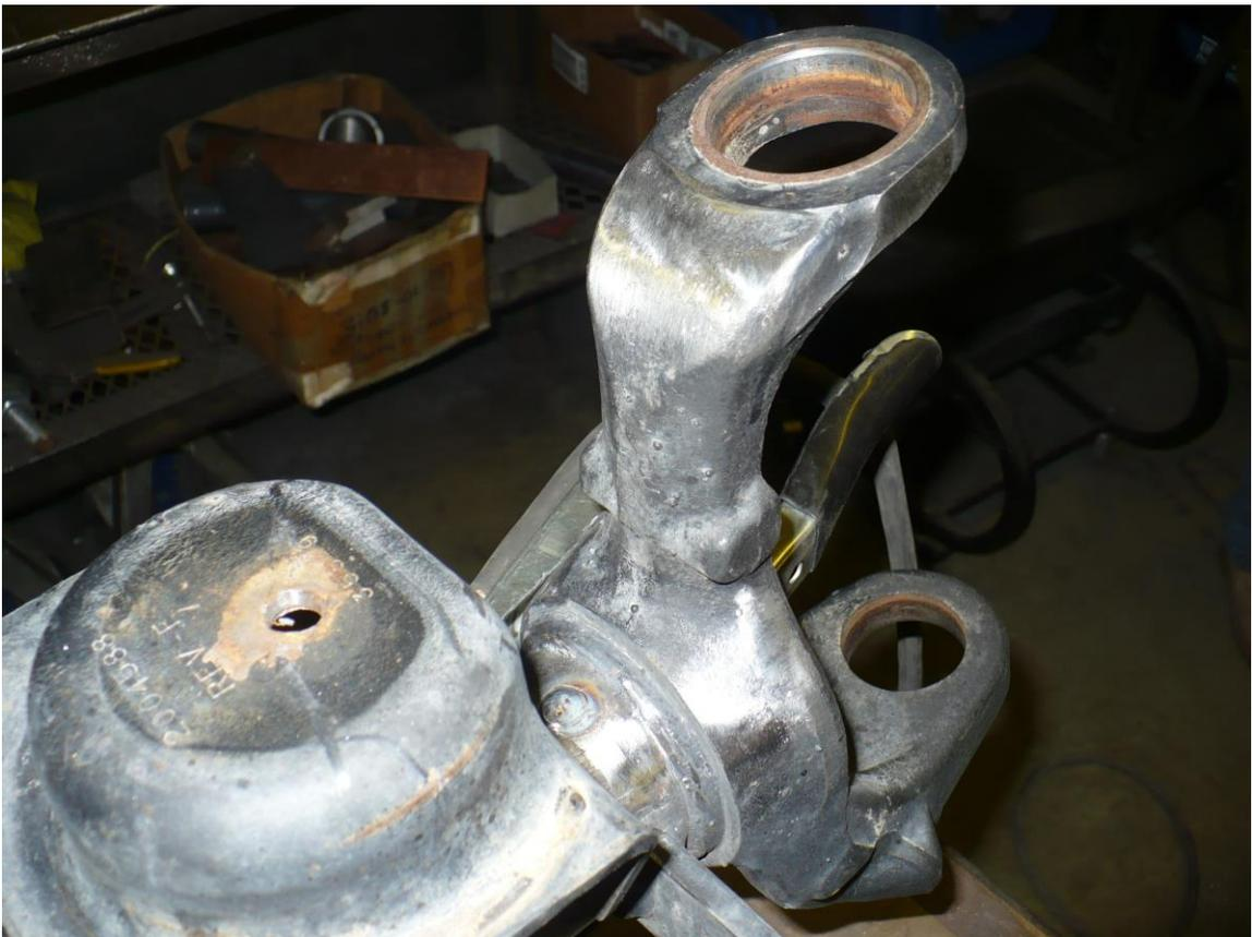
Once weld surfaces are prepared, place upper C-gussets in position. There will likely be a slight gap around the ball-joint area; use a C-clamp to tighten the gusset in the proper welding position.
