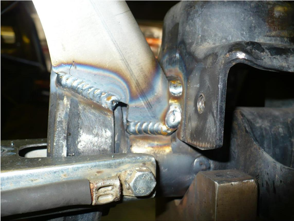
4. With upper C-gussets fully welded on, go ahead and move onto the lowers.
