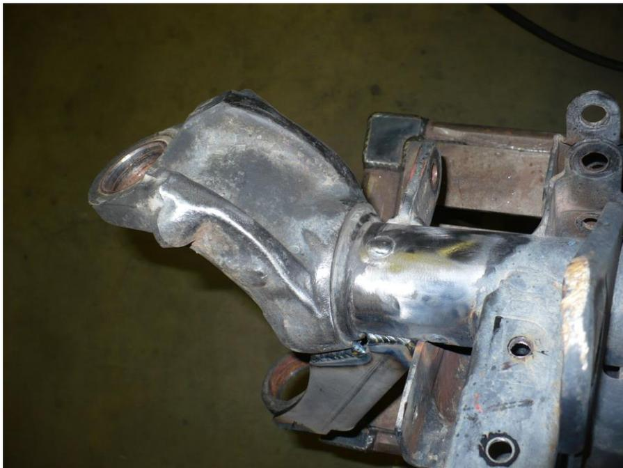
7. Tack the lower C-gusset on in several locations. We recommend tacking at the end of the weld for a clean weld. Once tacked, fully weld as shown in the pictures below.
