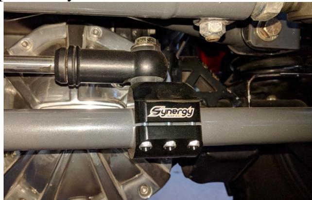
**Figure 3. Synergy 8003-20 Clamp Installed On Tie Rod**
