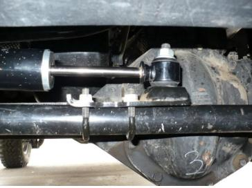
Figure 2. Factory Tie Rod Bracket 'Flipped'
