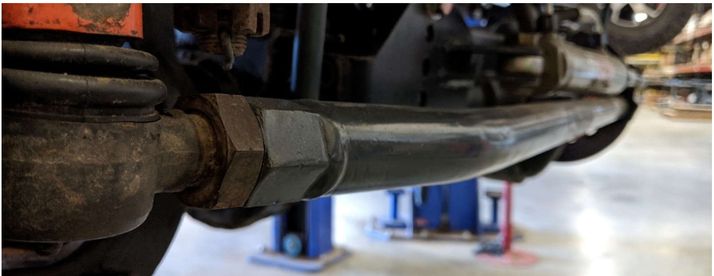
Figure 1. Tie Rod Installed with Bends Flat and Forward
