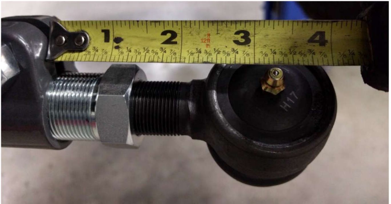
Figure 2. Maximum Length on Double Adjuster (Passenger) Side
