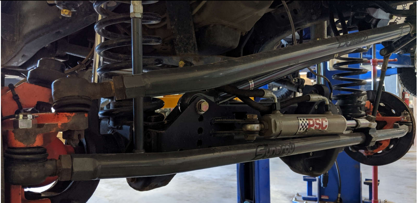
Figure 3. Tie Rod Correctly Installed
