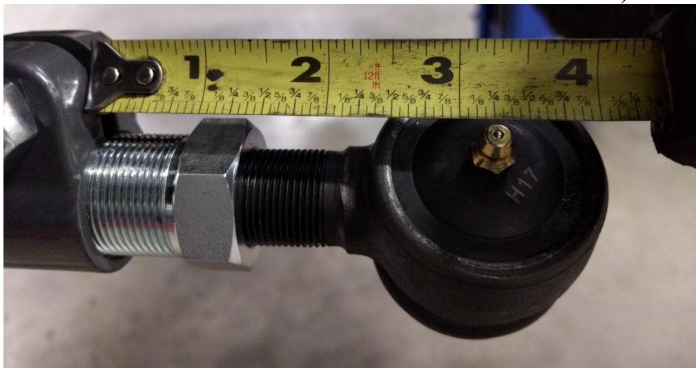
Figure 6. Minimum Thread Engagement on Pitman Arm Side of Drag Link
