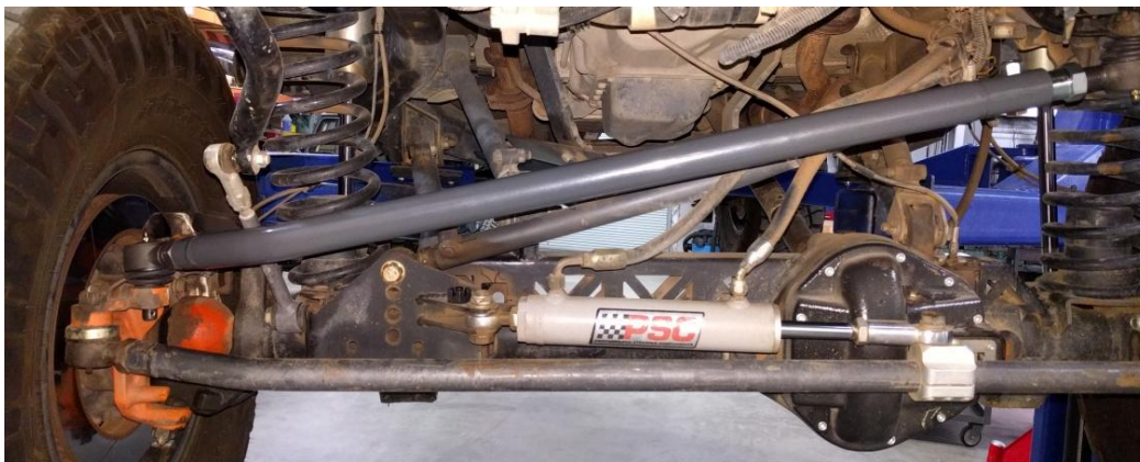
Figure 8. CORRECT Orientation of Drag Link
