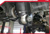
Install the lower end using the factory hardware and torque to 100 ft. lbs.
