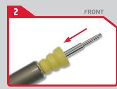
· Orient and install the bump stop onto the shock shaft as shown.
