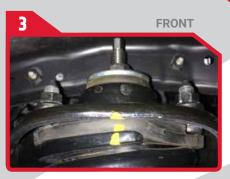
Before removing the strut assemblies mark the coil spring, spring isolator and strut tower to ensure the spring is reinstalled correctly.
