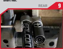
Install the upper end of the rear Falcon Shocks. Torque to 77 ft. lbs. (105 Nm).
