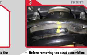
mark the coil spring, spring isolator and strut tower to ensure the spring is reinstalled correctly. The spring must be reinstalled in the same orientation that it was removed.
