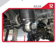
Install the lower end using the factory hardware and torque to 100 ft. lbs.
