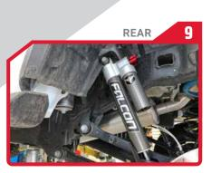
Install rear shocks with shaft down Shock #1= driver side Shock #2 = passenger side
