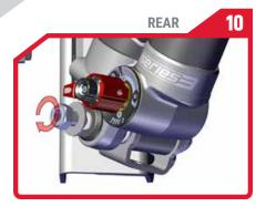
Install the provided hardware and torque to 40 ft. lbs.
