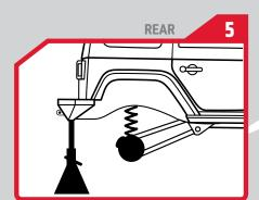
With the rear suspension at full droop remove the rear tires, and factory shocks.
