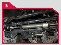
· Adjust stabilizer length by turning the wheel until the steering stabilizer eyelet fits into the bracket and aligns with the bracket holes. Using the softest setting to make the adjustment easier
