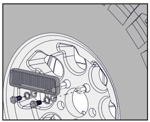
Install spare tire using the two included custom lug nuts as shown.
