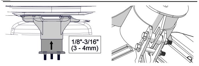
Remove the mount from the tire. Reinstall mount plate onto mount base.
