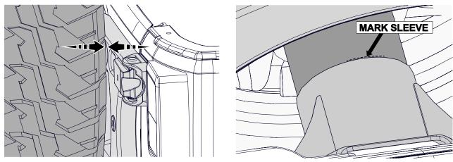
Slide the mount into the base on the tailgate. Push the tire firmly up against the cast hinge.
