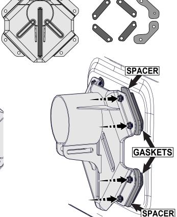
Apply thread locking compound to original bolts and install tire mount base as shown. Torque the 8 mounting bolts to 20 N-m (15 ft-lbs)
