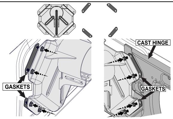
Place gaskets between tailgate and mount, apply thread locking compound and loosely install 4 of the original bolts
