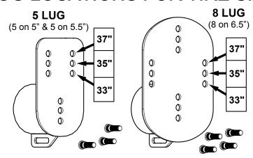
Press the included wheel studs into the appropriate set of holes for your tire size (3 wheel studs for 5 lug and 4 for 8 lug).
