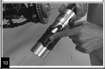
Apply pressure on the SpeedBump to make sure that it is completely seated and install retainer clamp. **Torque to 74.5 in-lbs (8 N-m)** and reinstall the factory isolator.
