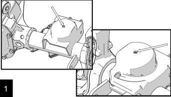
Reinstall the springs and the 467125 Speedbump Bumpstop at the same time so the spring is easier to install.
