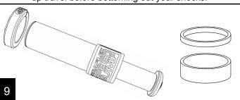
Coat the lower portion of the SpeedBump with black RTV silicone to help with noise and corrosion. Slide the bump stop into position.
