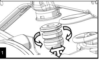
NOTE ORIENTATION: The upper SpeedBump cup snaps onto the frame bumpstop bell. Align the SpeedBump cup with the frame. The notched cutouts on the top side of the cup index around the factory bumpstop frame bracket.
