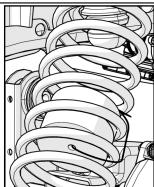
Install the #315 3/8" x 2" bolt through the bump stop and the #85 3/8" nut under the spring pad. Tighten bolt.
