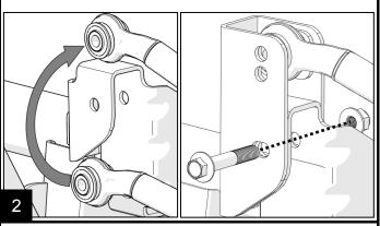
Install track bar bracket with the provided M12 bolt and M12 nut into the holes just drilled.
