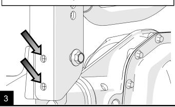
Install provided M14 bolt, spacer, and M14 nut into track bar relocation bracket and mount.
