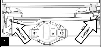
Mark the location for both holes to be drilled. Remove the bracket and drill a 1/2" hole in both locations.
