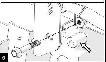
Place the track bar on top of the track bar mount. Temporarily install track bar relocation bracket onto the factory track bar mount with provided M14 bolt and nut.
