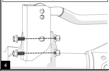
Install track bar onto relocation bracket using provided M14 bolt and nut. The lower position is for 2.5 - 3" lifts and upper position is for 4" lifts. Torque provided M14 bolt to 150 ft-lbs. [18mm & 21mm] Torque frame side track bar bolt to factory recommended specs. [21mm]
