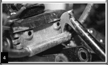
Remove the bump stops from the upper spring buckets.
