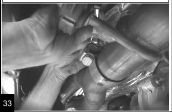
Using a chisel, remove the spot welded indexing stop on the intermediate pipe. This will allow the intermediate pipe to slide into the y-pipe to provide added clearance.
