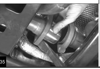
Install the supplied bolts into the exhaust flanges and tighten evenly. Make sure the exhaust pipes are still properly aligned and the spacers are straight. Check the exhaust system for clearance and retighten the Y-pipe clamp.
