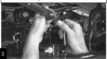
Unclip the ABS lines, and extend the breather tube by sliding the tube retainer clip down the shock tower 3". This will prevent the tube from being pulled tight during full axle droop.
