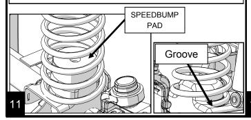
Install a bolt through the pads with the nut below the spring pads.
