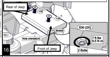
**IMPORTANT NOTE!** Due to clearance issues with the bumpstop pad on the axle it is important to have the frame side factory trackbar bolt installed from the front, and the nut to the rear.
