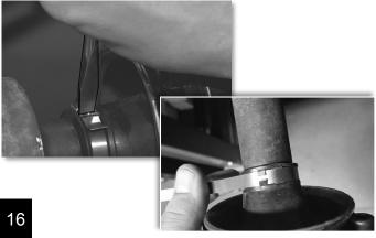
Reinstall the driveline. With the new wider flange, you will need to go around the bolt circle several times threading the bolts in a little at a time to avoid damaging the flange.
