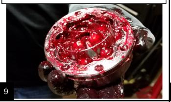
Use brake cleaner on a rag and clean the seal surfaces and bolt holes (shaded areas) of grease.
