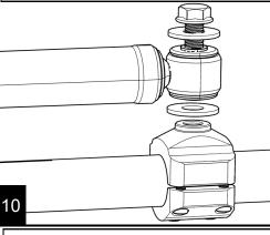
If you are not relocating your steering stabilizer, skip this step. Use an 18mm to tighten the sleeve nut.
