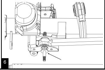
Install the body end of the stabilizer onto the stud and install the sleeve nut through the stabilizer bushing.
