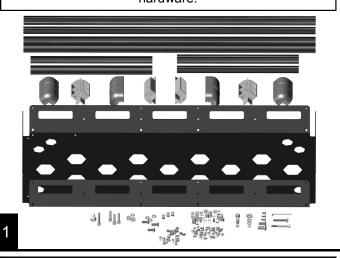
Loosely attach the Passenger Side Bracket(3) to the Rack Pan(5) using four M6x12mm bolts(20) and four T-nuts(14).
