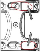
Loosely install the remaining three M8 bolts(24) and washers (17) for Drivers Side Bracket and the other 1/2" bolt(23) for the Passenger Side Bracket.
