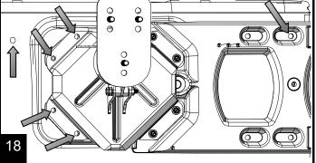
Clean off the surfaces of the tailgate and tire carrier before installing the Alta Cargo Rack. Also remove any plugs or accessories from the passenger most side holes in the Tire Carriers body.
