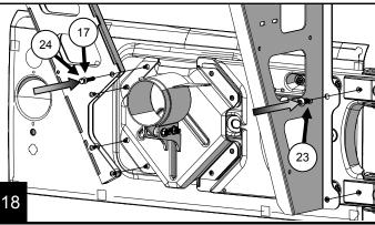
Install the Passenger Side Inner Bracket Brace and spacer(13) by first installing the M8x65mm bolt(25) and washer(17) into HD Carrier. Then install two 3/8" bolts(22), lock washers(16) and nuts(11) through the Passenger Side Bracket and Brace.
