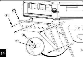
Loosely install two 3/8 bolts(22), washers(16) and nuts(11) through the Front Brace(2) and Passenger Side Bracket (3).
