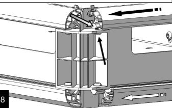
Prior to installation of final corner support, remove one of the short top rail to rack pan bolts closest to the end, then position 4 T-nuts(14) in the side rails. Place the corner support into position and reinstall the rack to rail bolt.
