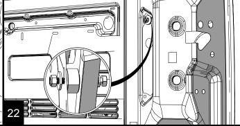
Tighten the bolts to the tailgate, (1st) starting with the four bolts(24) around the Adjustable Tire Carrier Mount Assembly attaching the Alta Rack's driver side Bracket, then (2nd) the two bolts(23) attaching the passenger side bracket to the HD Hinged Tire Carrier. Lastly (3rd) tighten the bolts(25) with the spacers and also the two bolts(22) and nuts(11) attaching the Passenger Side Brace to the Passenger Side Bracket.
