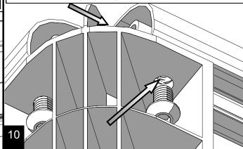
Now that all the corner supports are in place and all hardware lightly snug, square up the side rails and tighten down the bolts that hold the rail(6 & 7) to the rack pan(5). Four bolts on the short sides and eight on the long sides.
