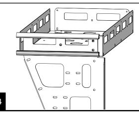
Apply Thread Locker to the end of the bolts and install M6x10mm bolts(19) and T-nuts(14) that hold on the other 2 short(7) and 4 long (6) side rails. There are eight holes on the long sides and four on the short. Leave T-nuts loose so side rails can slide on and slide them on. Snug up the side rails with the supplied 4mm allen wrench, leaving some play in the rails.
