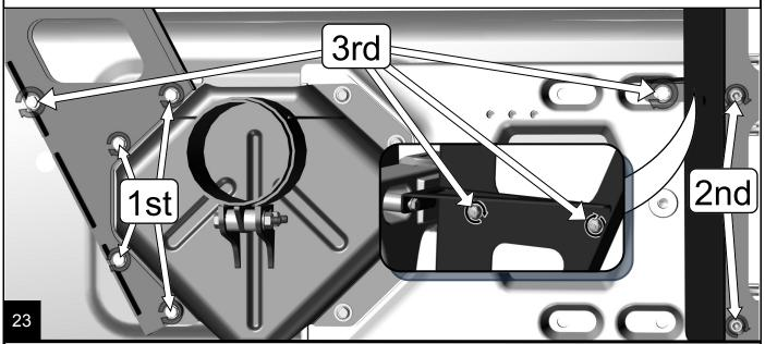
Now all that needs to done is to tighten all the bolts that attach the top Rack Pan to the Driver, Passenger and Front Brackets. Use steps 13 through 16 to help locate this hardware.
