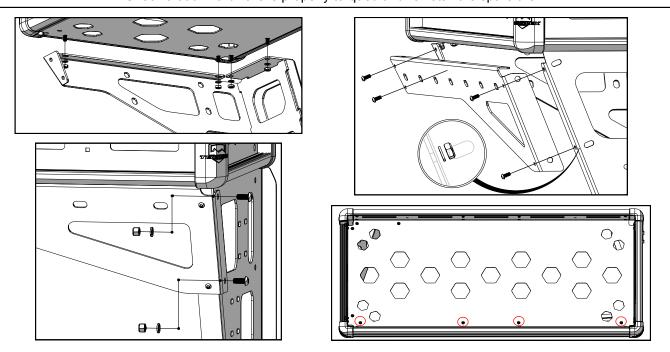
Re-torque all hardware after the first 300-500 miles of driving.
