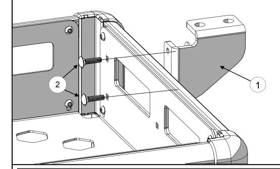
Install the CB Antenna Mount(1) onto the two 1/4" carriage bolts(2). Install 1/4" washers(4) and lock nuts(3) onto the 1/4" carriage bolts. Tighten nuts and torque to 7 ft-lbs (9 N-m). Install CB antenna (per manufacture's instructions) into one of the top two holes in mount.
