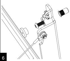
The top right hole on the tailgate uses the longer #727 nutsert. Thread the nutsert onto the tool.
