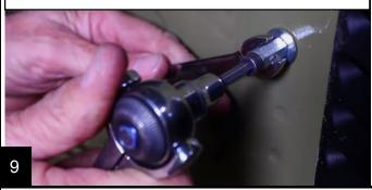
Install the table by threading the included mounting screws into the nutserts. Be sure to install the aluminum spacers on the top mounting screws.
