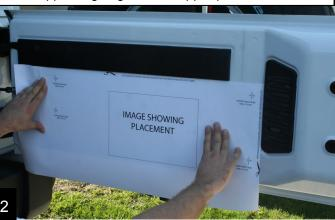
Tape the template in place and use a center punch to mark the four mounting hole locations.
