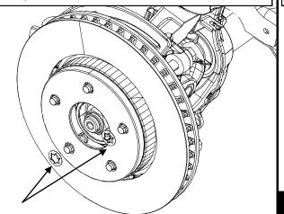
Install the new rotor. If slotted rotors are being used, the slots should be oriented as shown, with opposite side mirrored.
