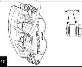
Repeat process on opposite side. Bleed brakes according to standard procedure.
