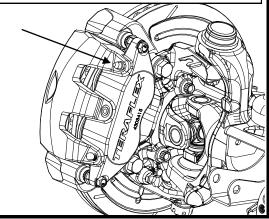
Remove one of the pin bolts from the TeraFlex caliper. Use a 14mm for the bolt and a 17mm to hold the pin.
