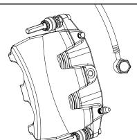
Install the brake line onto the new caliper using the factory banjo bolt and 2 new copper washers. Torque bolt to 23 ft-lbs (31 Nm) Note: Position of copper washers in relation to brake line
