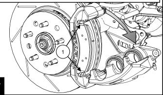
Swing the new caliper back into position and reinstall the pin bolt. Torque to **26 ft-lbs (35 Nm)**
