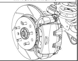
Remove the brake line from the factory caliper by removing the banjo bolt with a 15mm. Hint: Try to have your new copper washers ready so that this and the next step goes quick and easy, minimizing the mess.
