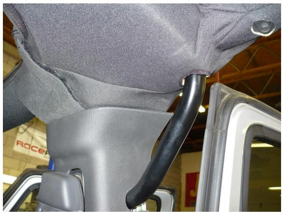
7. Notch the B-pillar trim as shown. A PDF template is included, cut the template out with scissors.
