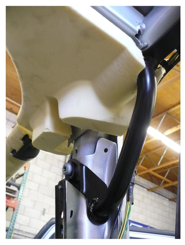
6. Remove the grab handles, zip the side bar padding up and insert the grab handle thru the cut hole as shown. Secure the upper grab handle bracket using the speaker pod bolts, do not fully tighten yet. Secure the lower bracket of the grab handle under the seat belt turning loop height adjuster and torque to 30 ft-lbs. Remove the speaker pod bolts and install the speaker pod and tighten the screws to 7 ft-lbs
