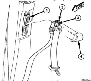
2. Remove the upper B-pillar trim panel (1) by pulling toward the center of the vehicle. The panel is secured with push in retaining pins (2)
