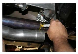
5.Carefully remove the front upper & lower and rear lower control arm mounts from the frame with a cutoff tool or torch. Be careful not to cut into the frame. (Figure 2)
