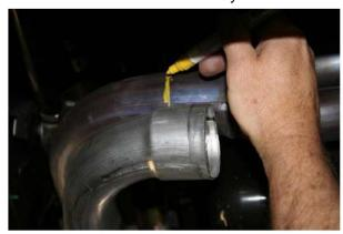
Cut the exhaust at your mark near the front corner of the oil pan, and remove the rest of the exhaust system including the catalytic converter, muffler and tailpipe. Be very careful to avoid damage to the oxygen sensor and wiring. Make the second cut on the exhaust where you made the mark a few inches in front of the catalytic converter and reinstall the exhaust at step 26. When you have the new muffler and tailpipe built and installed, have the exhaust shop weld in the front exhaust patch.
