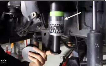
With the necessary shims in place, apply a coat of silicone sealant (not adhesive) over the cylinder of the Speedbump
