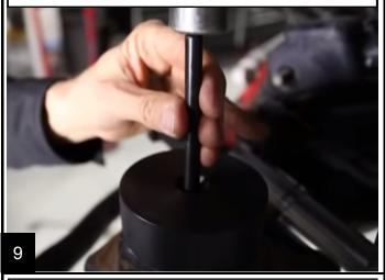
Drill a 3/8" hole; We recommend first drilling a pilot hole. Set the strike pad in place for measurements.
