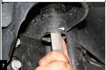
Slide the speedbump into place, check for a good fit between the speedbump and the cut factory tube.
