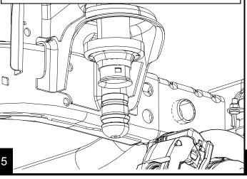
Measure down from the spring pocket 3.5" and mark the tube. Use tape as a straight guide for your cut. It is crucial that your cut is straight and square. Cut the tube.
