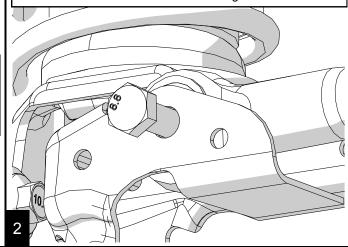
Disconnect the shocks from the axle with an 18mm.
