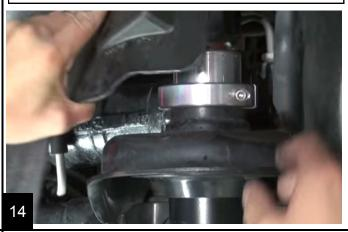
Install the springs and strike pad as an assembly. Install the 3/8" bolt (7/32" allen) into strike pad with the nut between the spring perch and the axle. Rotate the spring until it seats in the groove.
