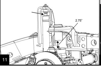
If the distance is 2.75" or less, remove the strike pad and adjust the speedbump with the provided spacers as required. If the distance is more than 2.75", use the provided spacers to lower the speedbump and adjust as necessary.
