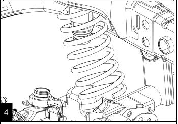
Remove the factory spring isolator. Remove the bumpstop by twisting and pulling to the side.
