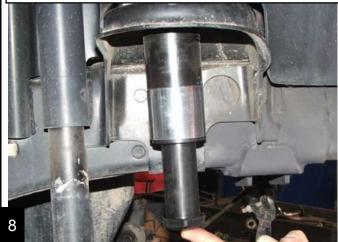
Remove the speedbump and center the strike pad on the spring perch. Use a center punch though the hole to mark the center.
