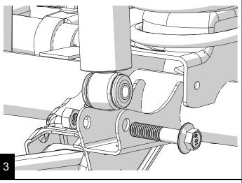
Lower the axle enough for the springs to be removed. Do not over stretch the ABS and brake lines.
