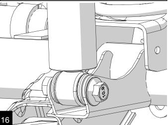
Reinstall the tires, torque lug nuts to 95-115 ft-lbs (128-156 Nm). Lower the vehicle to the ground and reconnect the track bar. Torque to 125 ft-lbs. Have an assistant turn the wheel back and forth to help align the track bar.
