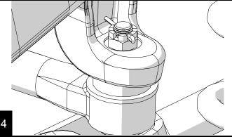
Loosen the nuts on the adjuster sleeve with a 15mm. Rotate the sleeve to adjust the track bar and center the axle under the vehicle. Torque nuts to 36 ft-lbs.
