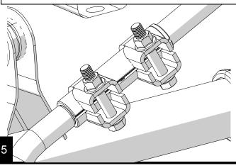
Using the supplied hardware, install the axle side of the trackbar with a 17mm. Torque to 40 ft-lbs.
