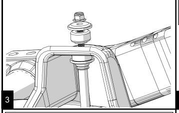
Reinstall the two lower bolts and nuts, torque to 21 ft-lbs.
