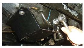
**Note:** Use flat washers to correct the spacing of skid plate when using stock bumper if necessary.
