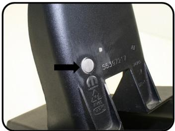
5. Use the factory screws to position the extension bracket as pictured. Use the holes closest to the middle of the extension bracket.
