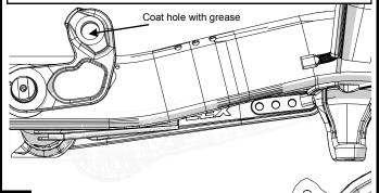
Position the arm as shown and slide it into place.
