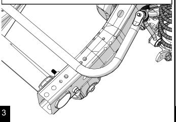
Remove the factory steering box bolt and replace it with the included 7/16" bolt. Apply thread locking compound and torque to 70 ft-lbs (95 N-m)
