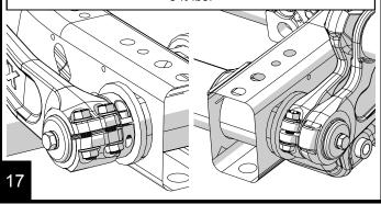
Using a small arbor press or vise, press the misalignment spacers into the rubber bushings of each sway bar link. Grease the inner diameter of the bushings and the outer diameter of the spacer to aid in installation.
