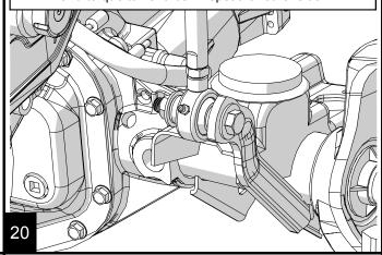
Lengthen the links so the forged sway bar arms are angled up slightly. The ends of the links are right and left hand threads. Simply twist the tube to adjust the length similar to a turn buckle. Adjust the link lengths so the engagement knob engages and disengages easily.
