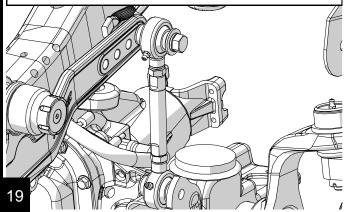
Install the lower link using the included 1/2"-13 bolts and stover nuts. Apply blue thread locking compound to the bolts and torque to 75 ft-lbs. Repeat for other side.
