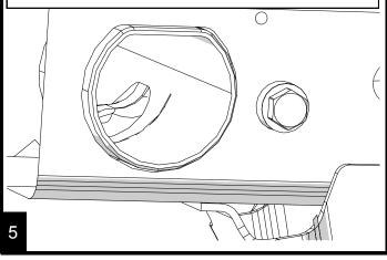
Coat the OD and ID of the frame bushing with grease. Orient as shown and drive the bushing into the front cross member using a dead blow hammer or rubber mallet.
