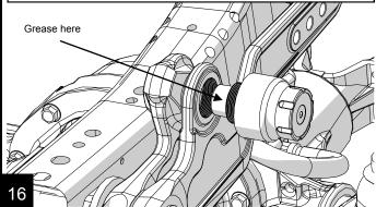
Install the three (Grade 8) 3/8" x 1 1/2" long pinch bolts in the arms. Don't forget the lock washers and blue thread locking compound. Alternate tightening the bolts on the right arm to equalize the load between the bolts. Final torque all pinch bolts to 50 ft-lbs. Torque the alignment spacer cap screw to 8 ft-lbs.
