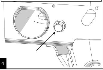
Ensure the ID of the front cross member is clear of debris and rust. Use a barrel sander to clean up if necessary.
